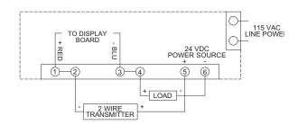
FIG. 3: FIELD WIRING FOR OPTION-LPS
